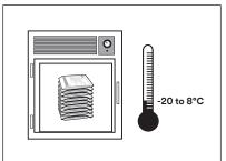
Store the unopened 3M Petrifilm Rapid E. coli/Coliform Count Plate pouches at frozen or refrigerated temperature equal to -20 to 8°C (-4 to 46°F). Use before expiration date on package. Just prior to use, all unopened pouches to come to room temperature before opening.
